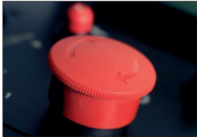
Activation of the stop button puts the system in a safe stop mode within 0.5 seconds.
