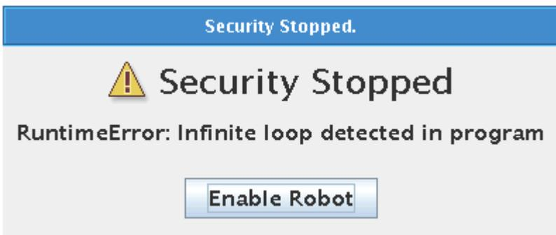
If you get this error messages is because the robot does not like to be caught in an Infinite loop. In this case the Thread program might be Infinite if the "var\_1" never change.
