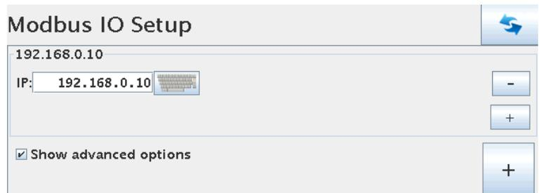
Key in the IP address of the Modbus node and press "OK".
