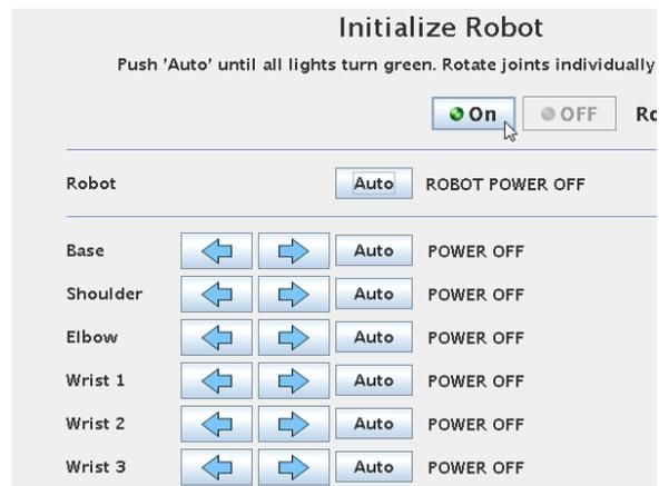
Press the “ON” button to turn on the power to the robot.
