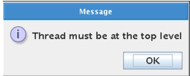
Here we got an error messages because the Thread has to be at top level. So we have to move the cursor position up and highlight "Robot Program" in our program tree.
