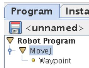
Notice how a “MoveJ” and “Waypoint” has been inserted and it starts looking like a program tree. The statements are still yellow because we have not defined the position of this Waypoint. MoveJ is the default and that’s why this is automatically chosen for us here. Later MoveL will be explained.
