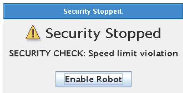
The robot started to move from Waypoint\_1 towards Waypoint\_2 in a straight line, but when the physics was in the way the robot showed the phenomena about increasing in speed and then rapid security stopped with "Speed limit violation" and never reaches Waypoint\_2.
