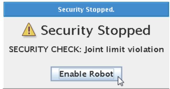
If you turn the joints all the way and beyond its limitation you will see an Error messages "Joint Limit Violation" which is a safety stop in order not to spoil the inside of the joint. Press "Enable Robot" to acknowledge the error messages.
