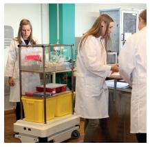
MiR100 can be outfitted with various modular solutions depending on the type of goods or materials needed to transport.
