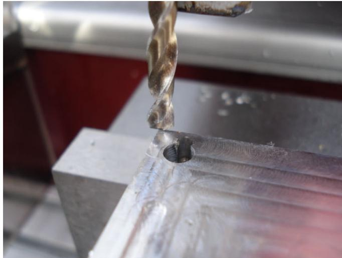
This is a practical but inaccurate way to measure the Zero point of the work-piece, because it is an eye approximation. The error is big compared to what some measuring tools out in the market can eliminate. For precise cutting, this method is not recommended, but since this is a beginner's course, it will do just fine.
